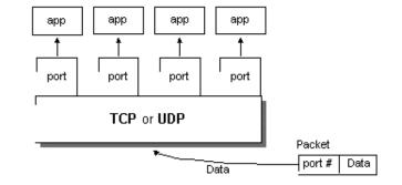
The UDP protocol provides for communication that is not guaranteed between two applications on the network. UDP is not connection-based like TCP. Rather, it sends independent packets of data, called **datagrams**, from one application to another. The order of delivery is not important and is not guaranteed, and each message is independent of any other.
